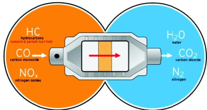
Figure 2: Harmful engine emissions enter the catalytic converter and exit as water vapor, nitrogen and carbon dioxide[4].
