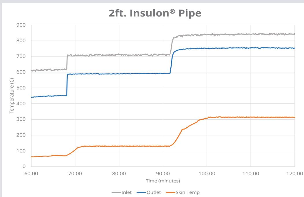
Figure 4: Insulon® case study showing temperature drop across two foot tube wrapped with Insulon and the skin temperature mid-length of the tube on the outer surface.
