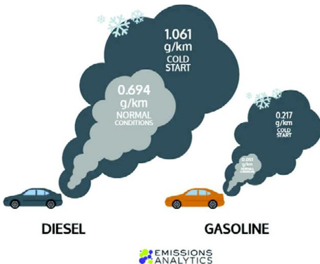
Figure 1: An illustration of NOx emissions during and after a cold start [2].
